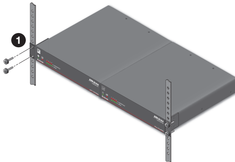
Figure 6. Secure Connected XPA Ultra Amplifiers to Rack
