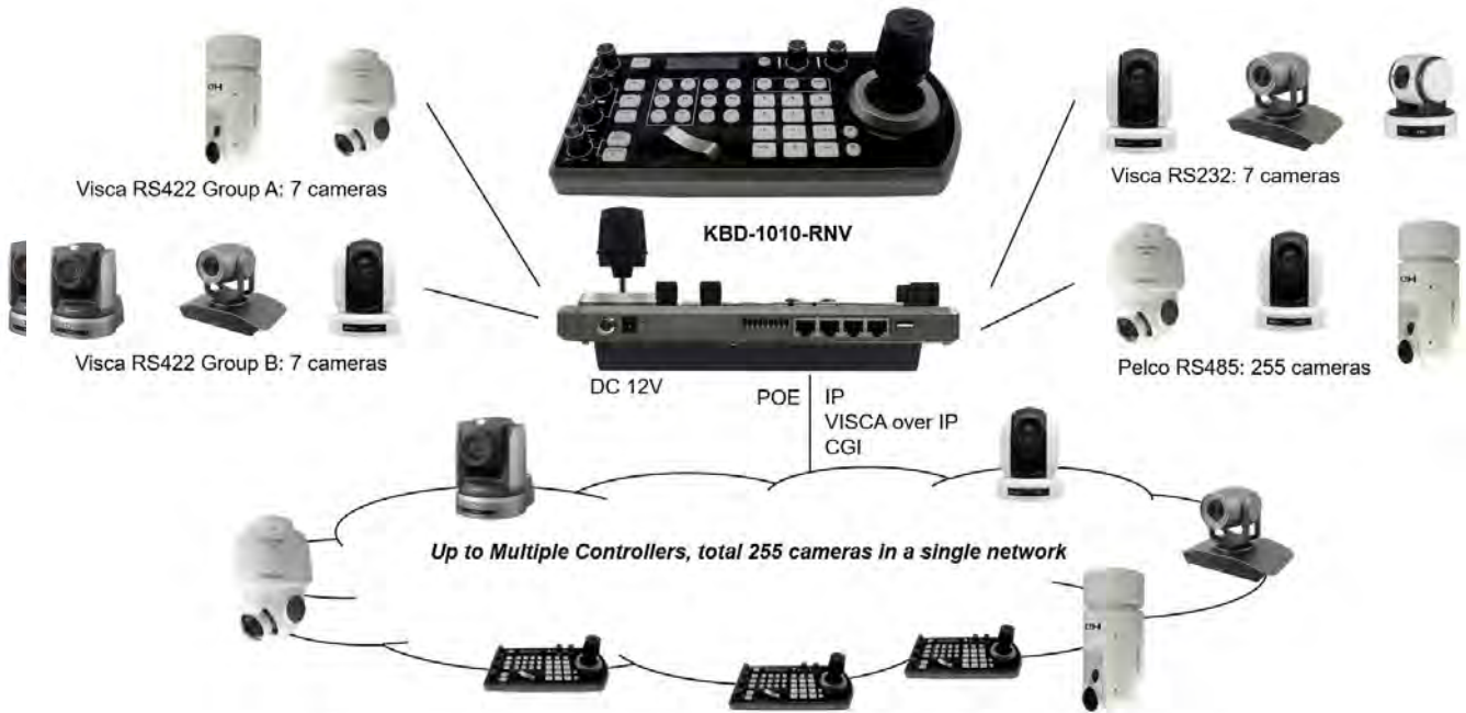
Cross Protocol Mix-control with RS232/RS422 and IP in one single system
