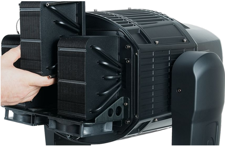
6. Unclip the center heatsink module safety cable.
